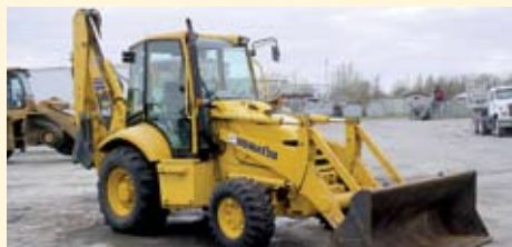
KOMATSU WB140-2 TRCTR LDR BACKHOE, S/N A20008, (ID 12554)WITH CAB, 4 WHEEL DRIVE, EXTENDABLE STICK, JOHN DEERE BACKHOE STYLE CONTROLS, 1.25-CU.-YD. LOADER BUCKET WITH BOLT-ON CUTTING EDGE, LEFT REAR VIEW MIRROR, DRIVE SHAFT GUARD, ADDITIONAL 375-LB. FRONT COUNTERWEIGHT, ENGINE BLOCK HEATER. . . . . $52,000
