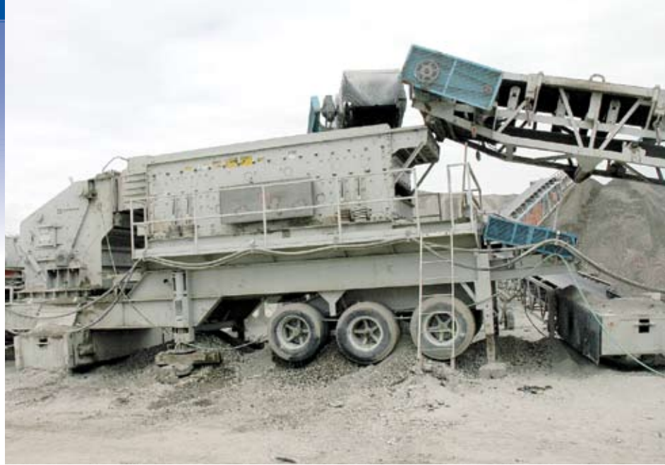
Gordon Schoonover and his crews at Zircon count on productive and reliable crushing and screening equipment from General Equipment. This new 425-horsepower Lippmann 4248LP closed-circuit impactor plant has a 62'x10' double-deck screen and a 36-inch permanent magnet. Crews were recently using the plant in Mapleton, N.D., to recycle concrete and asphalt from a demolition job for use as road base and backfill material.
