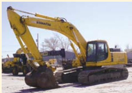
KOMATSU PC300LC-6 HYD EXCAVATOR, S/N A84742, (ID12701) WITH 21'3" BOOM, 13'2" ARM, 33.5" TRIPLE GROUSER TRACK PADS, CAB WITH HEAT AND A/C . . . . . $139,000
