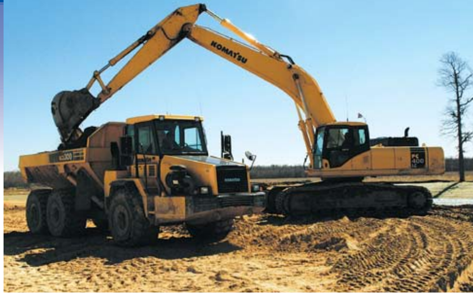
As the excavator/articulated dump truck combination gained widespread acceptance in the last decade or so as a cost-effective method of moving dirt, Komatsu introduced a highly regarded line of articulated haulers.
