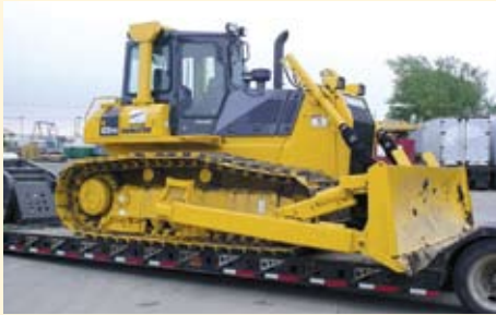
KOMATSU D65PX-15 CRAWLER TRACTOR, S/N 67721, (ID 12593) POWERED BY 190-HP DIESEL ENGINE, EQUIPPED WITH HYDROSTATIC STEERING SYSTEM, PALM COMMAND CONTROL SYSTEM WITH ELECTRONIC CONTROL, 36" SINGLE-GROUSER SHOES, POWER TILT AND PITCH DOZER ASSEMBLY, RIGID DRAWBAR, STEEL CAB WITH A/C, HEATER, DEFROSTER, PRESSURIZER, FABRIC SUSPENSION SEAT, LUNCHBOX HOLDER, AM/FM RADIO WITH CASSETTE, ADDITIONAL WORK LIGHTS ON FRONT AND REAR . . . P O R
