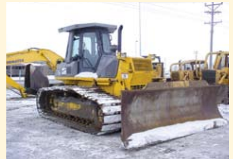
KOMATSU D61PX-12 CRAWLER DOZER, S/N 1091, (ID 12421) WITH 6-WAY DOZER ASSEMBLY, RIGID-TYPE DRAW BAR, ADDITIONAL REAR LIGHTS, ROPS CANOPY, STEEL CAB W/ A/C, HEATER, DEFROSTER, PRESSURIZER, SUN VISOR/WATER SEPARATOR . . . . . P O R
