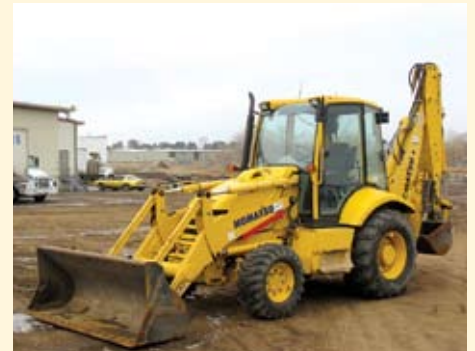
2003 KOMATSU WB140-2 TRACTOR LOADER BACKHOE, S/N A20008, (ID 12554) WITH CAB, 4-WHEEL DRIVE, EXTEND STICK, JD BACKHOE-STYLE CONTROLS, 1.25-CU.-YD. LOADER BUCKET WITH BOLT-ON CUTTING EDGE.....$49,000.00
