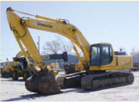
2001 KOMATSU PC300LC-6 HYD EXCAVATOR, S/N A84742, (ID 12701) WITH 21'3" BOOM, 13'2" ARM, 33.5 TRIPLE-GROUSER TRACK PADS, CAB WITH HEAT AND A/C.....$129,000.00
