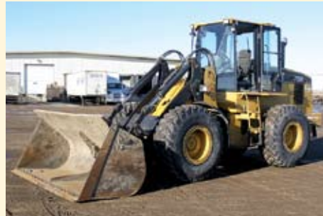
1997 CATERPILLAR IT28G WHEEL LOADER/ INTEGRATED TOOL CARRIER, S/N 8CR00348, (ID 13818) WITH CAT DIESEL ENGINE-105HP, ELEC. PS TRANSMISSION, WET-DISC BRAKES, 20.5R25 XTLA MICHELIN TIRES, CAB WITH A/C AND HEATER, RIDE CONTROL, BUCKET, FORKS AND JIB BOOM.....$72,000.00
