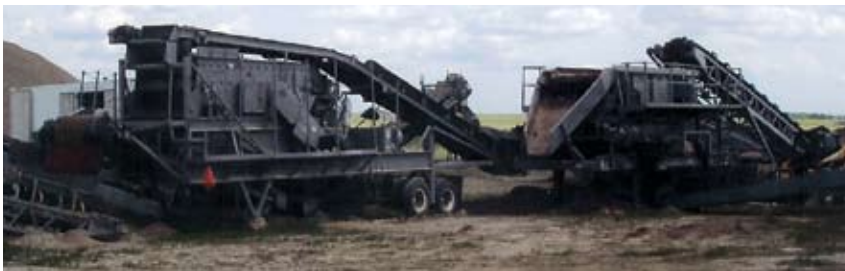
One of Farden Construction's primary pieces of crushing equipment is this Cedarapids 45-inch cone crusher.
