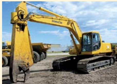
KOMATSU PC250LC-6L EXCAVATOR, S/N A80283, (ID 14108) WITH 19'4" ONE-PIECE BOOM, 31.5 TRIPLE-GROUSER SHOES, CAB WITH HEAT, 158-HP DIESEL ENGINE, APPROX 62,000 LBS, MACHINE EQUIPPED WITH LABOUNTY MSD40R SHEAR..... PACKAGE PRICE $109,000.00
