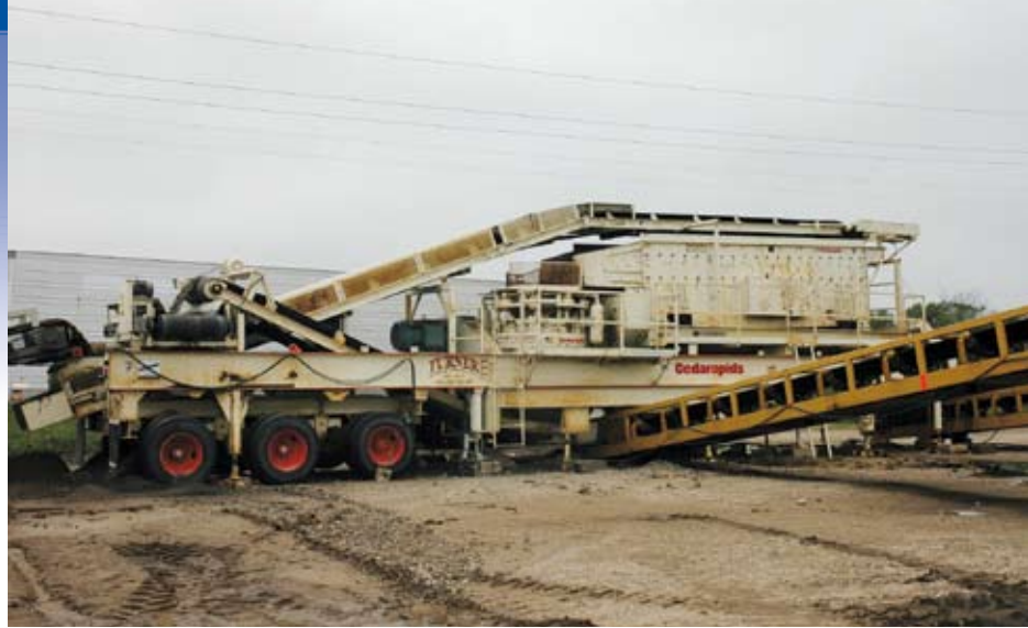
Turner Sand & Gravel relies on this portable Cedarapids cone crusher to crush nearly 200,000 tons of material each year, mainly Class 5 material it uses in its road regraveling operations.
