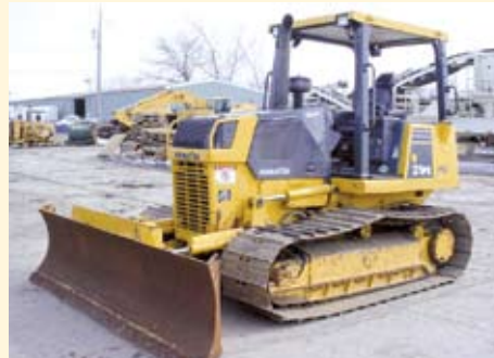
KOMATSU D31PX-21 CRAWLER TRACTOR, S/N 50126 (IDM00014012) WITH 6-WAY DOZER BLADE, OPEN ROPS, 75-HP KOMATSU SAA4D102E-2 DIESEL ENGINE, HS TRANSMISSION, 24" SHOES, APPROX 16,780 LBS.....$49,000.00
