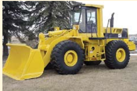
KOMATSU WA420-1 WHEEL LOADER, S/N 10166, (ID M00011155) WITH ROPS CAB, HEATER, KOMATSU 202-HP SA6D110-1 ENGINE, APPROXIMATELY 42,500 LBS., 26.5-25 TIRES, 4.25-CU.-YD. GENERAL PURPOSE BUCKET WITH BOLT-ON CUTTING EDGE, REBUILT ENGINE .....$49,000.00
