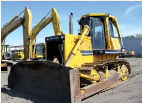
KOMATSU D85A-21 CRAWLER DOZER (ID M20222) WITH ROPS, CAB, A/C, HEATER, DEFROSTER, STRAIGHT-TILT DOZER BLADE, 24" PADS, RIGID DRAWBAR, AUX HYD FOR RIPPER, NEW UNDERCARRIAGE ..... $99,000.00
