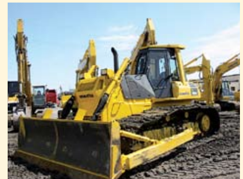
KOMATSU D65PX-12, S/N 65477 (IDM00013609) WITH CAB, A/C, HEATER, DEFROSTER, ROPS, STRAIGHT-TILT HYD BLADE, 36" SINGLE-GROUSER PADS, RIGID DRAWBAR ..... $169,000.00
