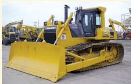
KOMATSU D85PX-15 CRAWLER DOZER (ID M14010) WITH DIRECT-INJECTED TURBOCHARGED AND AFTERCOOLED ENGINE, 75 AMP ALTERNATOR, STRAIGHT-TILT BLADE, ROPS, CAB W/HEATER, DEFROSTER, A/C AND PRESSURIZER, SUSPENSION SEAT, HYD FOR REAR ATTACHMENT, 36" SINGLE- GROUSER SHOES, FRONT AND REAR WORK, LIGHTS ON CAB, AM/FM CASSETTE RADIO, LARGE- CAPACITY BATTERIES, END AND CENTER GUIDES FOR TRACKS. .... $355,000.00
