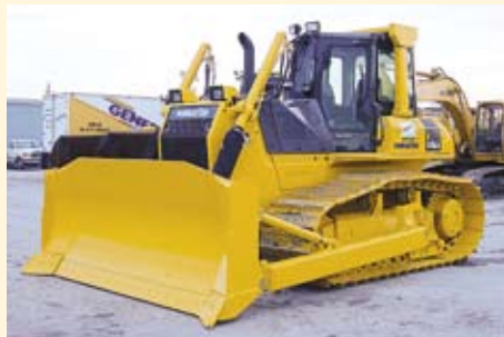
KOMATSU D65WX-15 CRAWLER TRACTOR (ID M13582) POWERED BY KOMATSU S6D125E-3 DIESEL ENGINE EQUIPPED WITH CAB, AIR, FABRIC SUSPENSION SEAT, AM/FM RADIO, 32" SINGLE-GROUSER SHOES, SEMI-U TILT DOZER ASSEMBLY, HYDRAULICS FOR REAR EQUIP, ADDITIONAL WORK LIGHTS FRONT AND REAR, KOMATSU 3-SHANK PARALLELOGRAM RIPPER. .... $175,900
