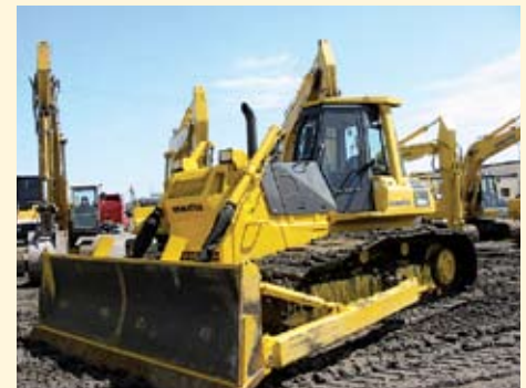
KOMATSU D65PX-12, S/N 65477 (ID M00013609) WITH CAB, A/C, HEATER, DEFROSTER, ROPS, STRAIGHT-TILT HYD BLADE, 36" SINGLE-GROUSER PADS, RIGID DRAWBAR ..... $169,000
