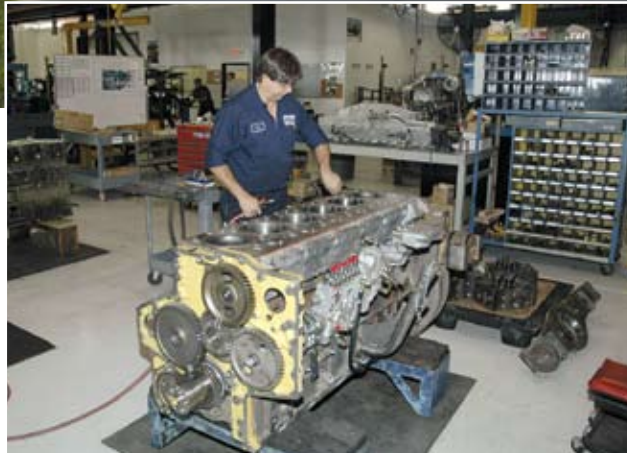
Located in Lexington, Ky., Komatsu Remanufactured Products employs about 140 people, including technician Paul Carrico, shown here assembling a reman engine for a D375 dozer. All reman engines are dyno-tested after final assembly.
