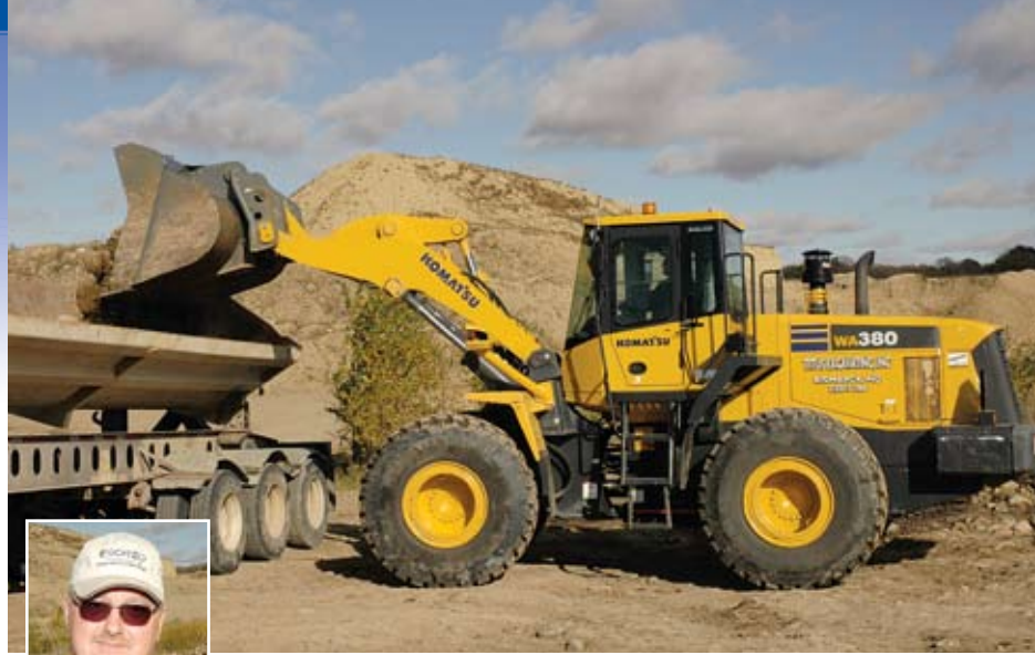
Titus Excavating Operator Cliff Heilman uses the Komatsu WA380-3 wheel loader to move a load of rock that will eventually be used for bank stabilization work.
