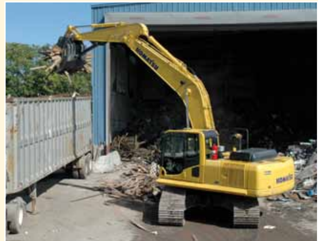
Komatsu’s new PC200LC-8 Waste Spec Arrangement is built for the rigors of waste handling in transfer stations, landfills and construction and demolition debris applications. Features such as wide core coolers keep the machine temperature down for better production even in the most severe environments.
