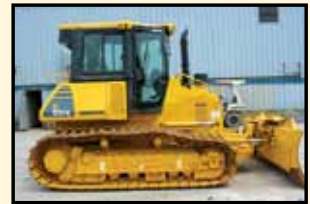
1 - 2008 KOMATSU D51PX-22 CRAWLER TRACTOR (E29118), POWERED BY A SAA6D107E-1 130-HP DIRECT-INJECTED TURBOCHARGED DIESEL ENGINE, 28" SINGLE-GROUSER SHOES, ROPS CAB WITH AC/HEAT/PRESSURIZER, KOMTRAX.....$135,000
