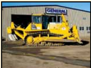
2010 KOMATSU CRAWLER TRACTOR D155AX-6 , S/N 80920 (E28273), 5 TURBOCHARGED & AFTERCOOLED DIRECT-INJECTED ENGINE, 36" EXTREME-SERVICE SHOES, 3-SHANK RIPPER W/VARIABLE DIGGING ANGLES, KOMTRAX.....$549,500
