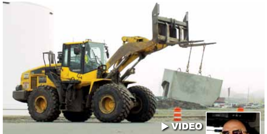
Sellin Brothers Operator Gaylan Sahlberg moves a concrete box with a Tier 4 Interim WA380-7 wheel loader at the West Fargo Main Avenue reconstruction project.
