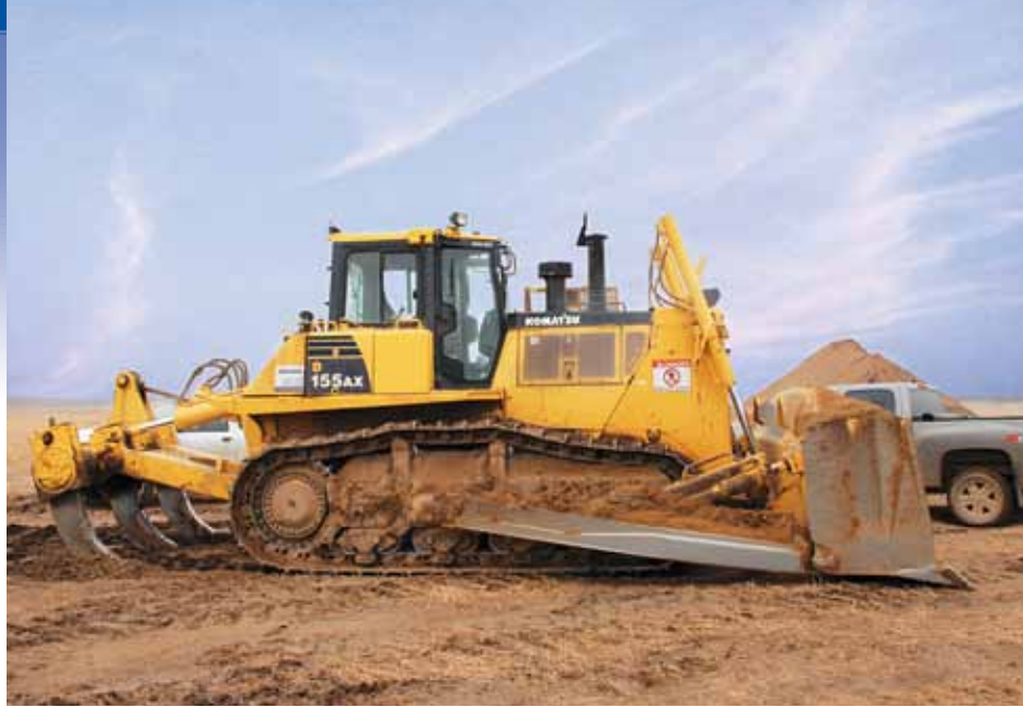
Edwards Gravel & Construction uses a Komatsu D155AX dozer to push up and maintain stockpiles. "There are times when we've crushed 24 hours a day, and the D155 has no problem keeping up," said Owner Robbie Edwards. "Its production and fuel efficiency lowered our per-ton costs."
