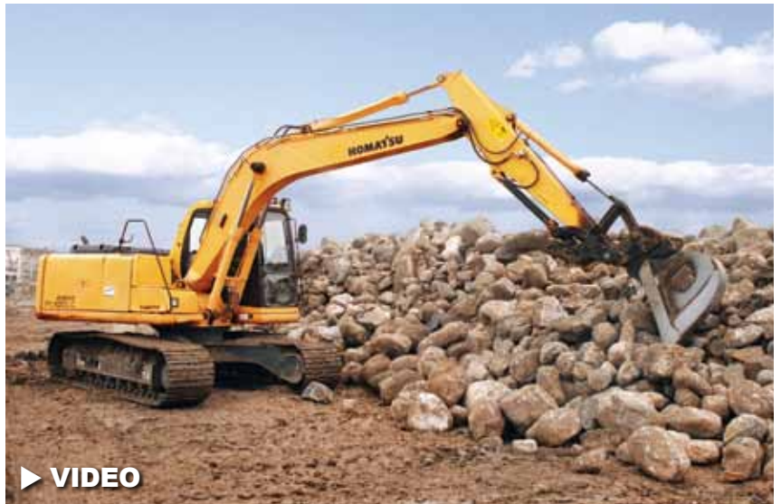
An Edwards Gravel & Construction operator uses a Komatsu PC120 excavator to pile large rocks at one of the company's leased pits. It also uses the machine for digging basements and trenches and for demolition work.
