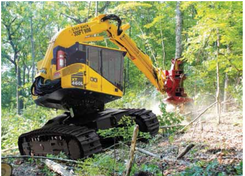
Four sizes of forestry tracked harvesters and tracked feller bunchers are produced at Komatsu's CMO, among them are new Dash-3 models, including the XT460.
