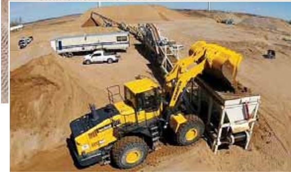
This direct-drive crushing spread designed for H&S Contracting includes Superior stackers, a KPI-JCI K200 cone plant and a Komatsu WA500 wheel loader to feed it. H&S purchased the package through General Equipment & Supplies. "General Equipment knows this industry better than anyone – it's that simple," said President Tracy Hazelton. "We were just getting into the industry, but they treated us like a big-time customer and designed this awesome plant for us."
