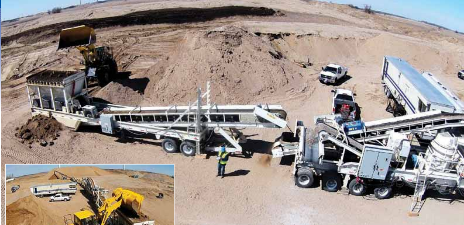
This direct-drive crushing spread designed for H&S Contracting includes Superior stackers, a KPI-JCI K200 cone plant and a Komatsu WA500 wheel loader to feed it. H&S purchased the package through General Equipment & Supplies. "General Equipment knows this industry better than anyone – it's that simple," said President Tracy Hazelton. "We were just getting into the industry, but they treated us like a big-time customer and designed this awesome plant for us."
