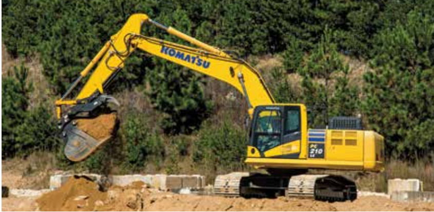
The 21-ton PC210LC-11 is the smallest excavator that Komatsu's Chattanooga Manufacturing Operation produces. The largest is the 49-ton PC490LC-11.
