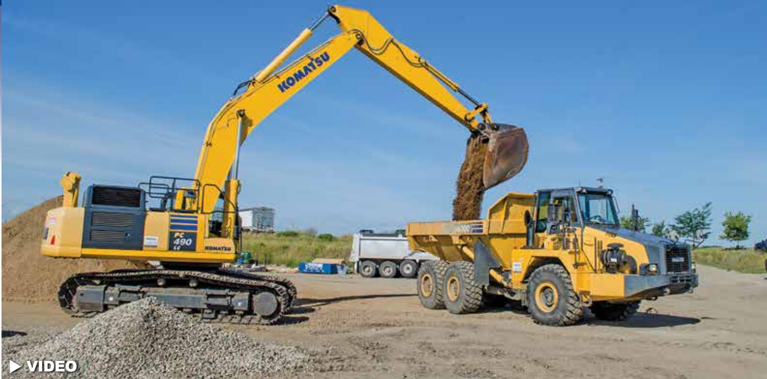
A Komatsu PC490LC excavator and an HM300 articulated truck move material at the site of a 36-unit apartment complex project.
