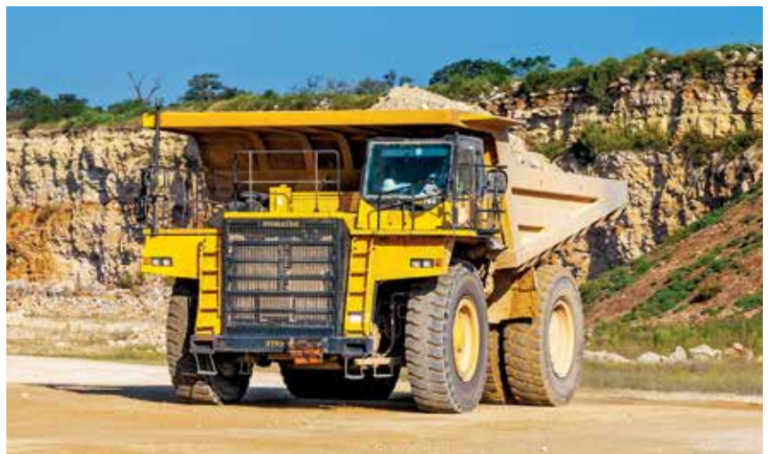
Komatsu's Peoria Manufacturing Operation produces seven of the largest electric-drive mining trucks in the world, ranging from the 200-ton-capacity 730E to the 400-ton 980E, as well as autonomous versions of some models.
