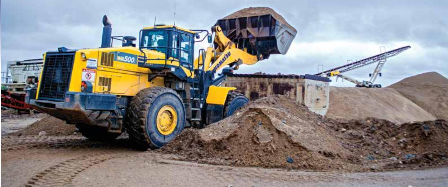
Using a Komatsu WA500 wheel loader from General Equipment & Supplies Co., a Turner Sand & Gravel operator feeds the crushing spread at the company's pit in Vergas, Minn.
