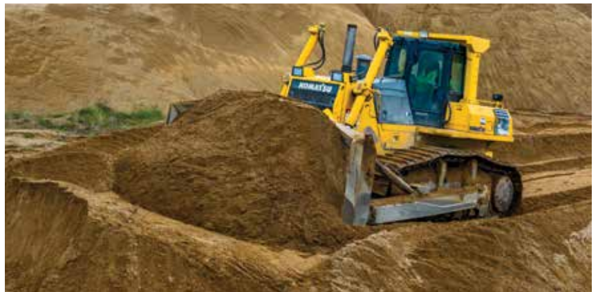
A Turner Sand & Gravel operator uses a Komatsu D155AX dozer to create a stockpile of sand for a future order.
