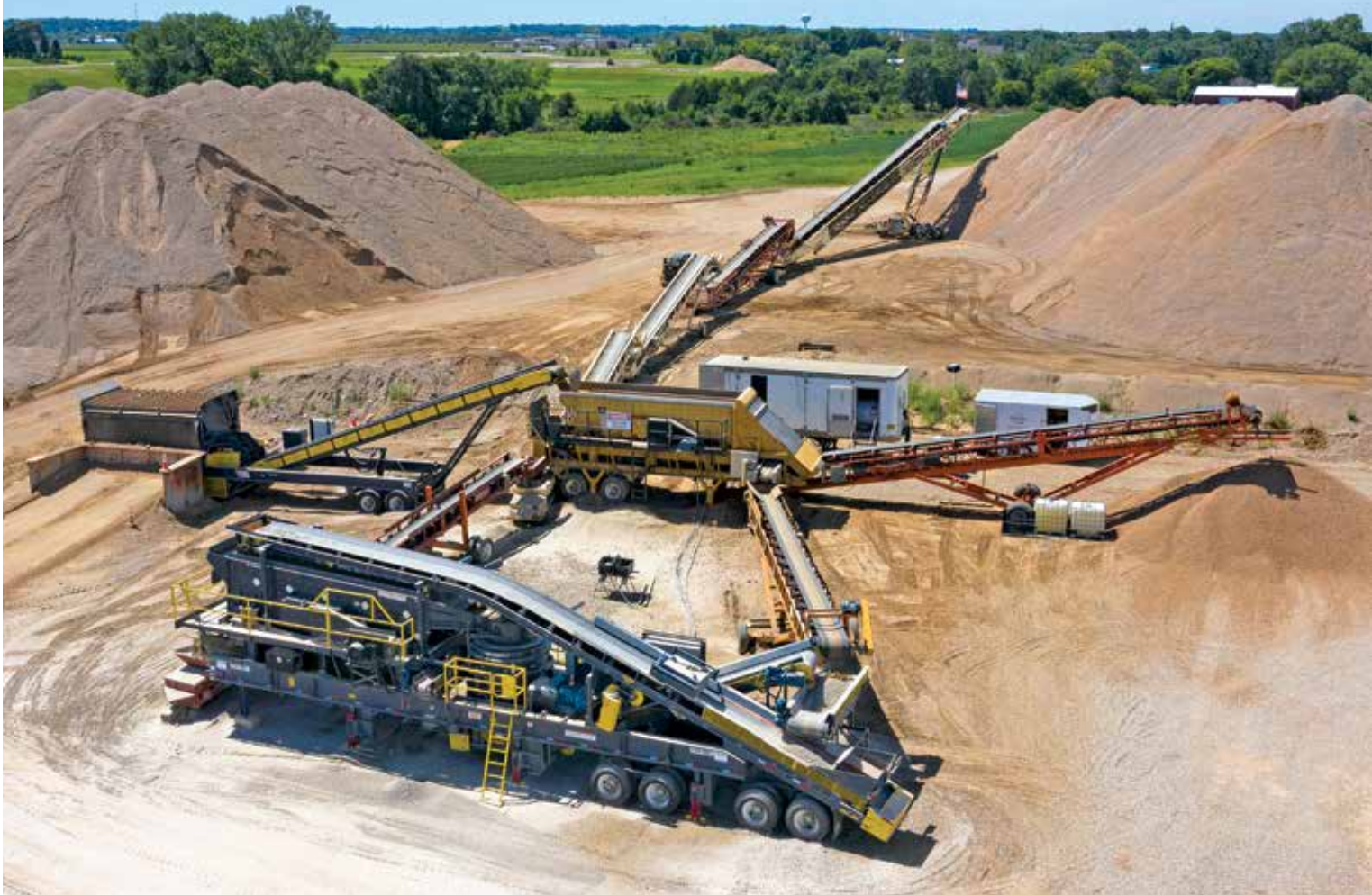
General Equipment & Supplies, Inc. helped Pentagon Materials outfit its new Maranda Pit in Belle Paine, Minn., with a state-of-the-art spread in March. It features a KPI-JCI/Astec 300 Kodiak cone crusher, a closed-circuit 300-horsepower plant with a 6-by-20-foot triple-deck Terex screen; a Vale 4218 double-belt feeder; and a Superior Industries stacker conveyor.
