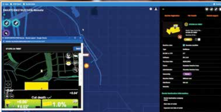
Project Surveyor Randall Hendra monitors Tomahawk Construction's Komatsu iMC machines as well as its Topcon-equipped machines from his desk with Smart Construction Remote. "Between tracking machines, uploading files and remotely supporting our operators, Smart Construction Remote paired with Komatsu iMC equipment has greatly increased our efficiency," said Hendra.
